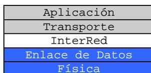
FIGURA 4-2. PILA DEL PROTOCOLO TCP/IP
