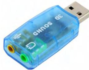
Fig 4.4 Tarjeta de audio USB implementada (3D Sound).
